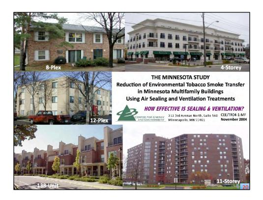
This slide shows 5 buildings studie by the Center for Energy and Environment in Minnesota. They investigated how much air infiltrated between neighboring apartments, and whether sealing and additional ventilation of smokers' units could decrease or eliminate SHS intrusion into nonsmokers' units. They concluded that these measures often reduced interunit airflows, but failed to eliminate SHS infiltration.
