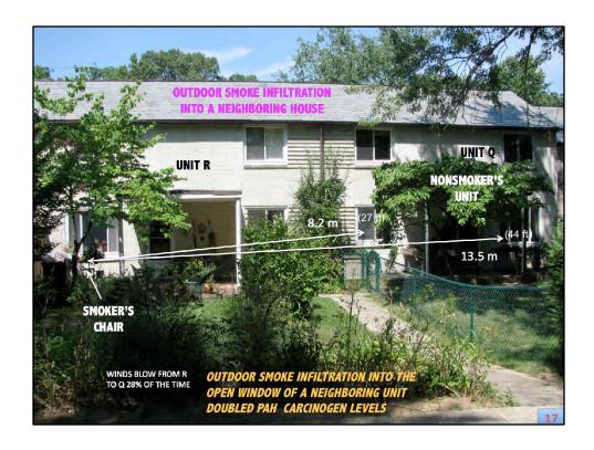
In a study of outdoor SHS penetrating thru open windows, a smoker smoked cigarettes for 20 minutes in the location denoted "smoker's chair" in the photo above. Real-time EcoChem PAS2000 CE monitors for particulate polycyclic aromatic hydrocarbons (PPAH) were located in the neighboring nonsmoker's units at 8.2(27 ft) and 13.5 meters (44 ft) distant respectively.
