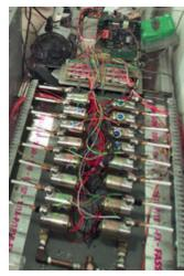
Researchers at the Berkeley Lab use this smoking machine to gauge how much nicotine from cigarette smoke is absorbed into drywall and other common surfaces.
